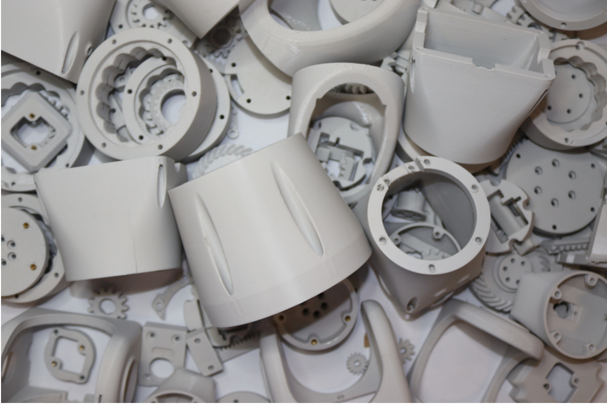
Figure 5: 3D printed prototype parts
